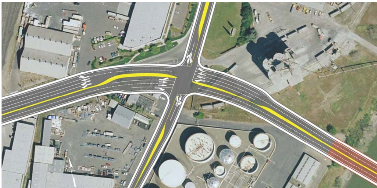
Figure 3. Alignment B, 15 th Street Connection Concept
