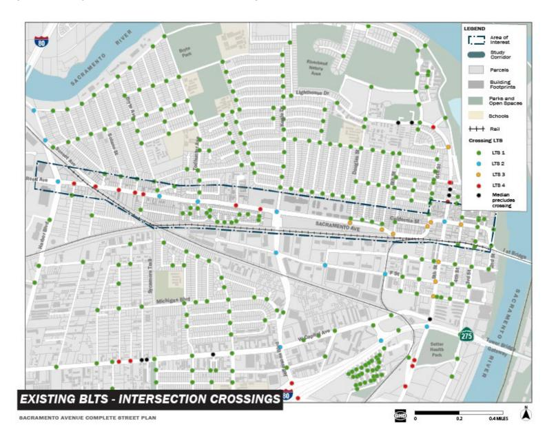
Figure 6 Bicycle Level of Traffic Stress – Overall
